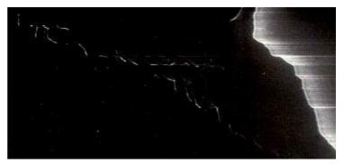
nonlinear space charge waves" - mystery lightning-leading waves. Those streamers then unite within a few milliseconds to form a closed plasma channel, the so-called 'leader'. This channel is it then that is transporting the charge of the main lightning, the stroke. But without the 'building blocks' of the streamers, no such channel can be formed.
